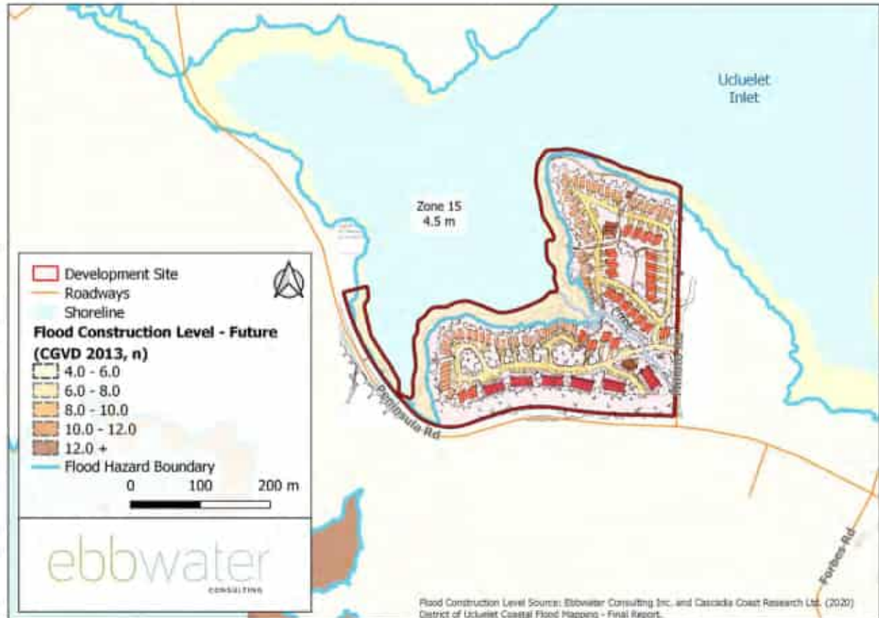
Figure 4-4: Coastal Storm Flood Planning Support Map for Flood Construction Level – zones for rare event (future - 0.5% Annual Exceedance Probability (AEP) + 1.0 m RSLR + 0.6 m freeboard) overlaid on the Draft Site Concept. Note that the Draft Site Concept georefer
